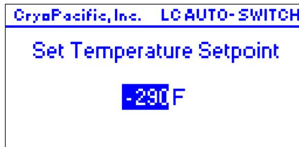
converting from Celsius to Fahrenheit, use  $^{\circ}\text{F} = (^{\circ}\text{C} \times 9/5) + 32$ . Press the  $\leftarrow$  key to save the setpoint. The factory default is  $-290^{\circ}\text{F}$ .
