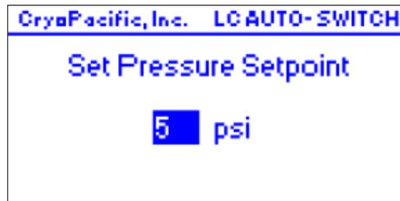
formula  $^{\circ}\text{psi} = \text{kPa} \times 0.145$ . Press the  $\leftarrow$  key to save the setpoint. The factory preset is 5 psi.
