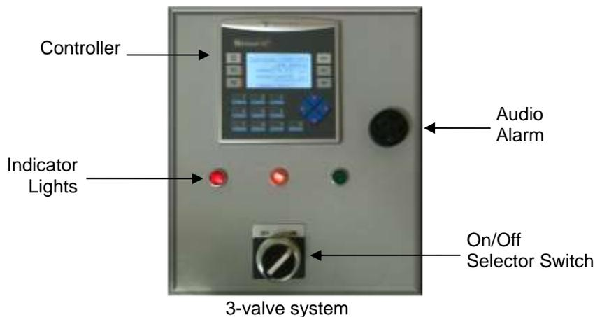
Indicator lights are located on the control panel underneath the controller screen. There is one indicator light for each solenoid valve (or intended cylinder) numbered from left to right 1, 2, 3, and 4. An audio alarm is located on the right side of the controller and has the option of sounding when all three cylinders are empty.
