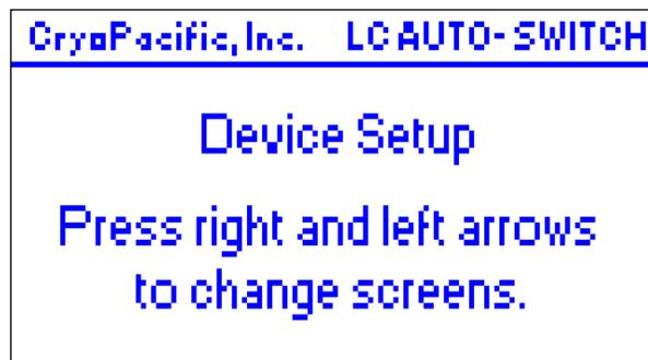
submit the password. The *Device Setup* screen will appear. Use the right and left arrows to scroll between screens. Press the ESC (escape) button on the top right of the controller to exit at any time.
