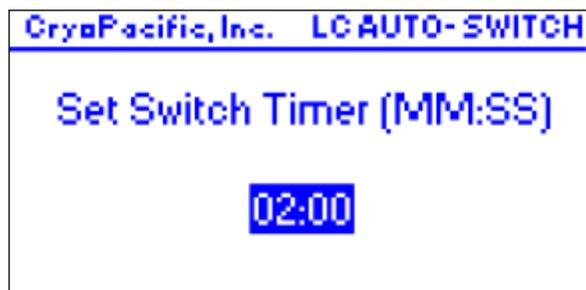
controller switches valves and waits the delay saved in the switch timer for the feed line to prime. When primed with LN<sub>2</sub>, the switch condition evaluates to false. The purpose of the switch timer is to prevent the system from rapidly switching through all the valves without giving the newly-switched cylinder enough time to prime the feed line.
